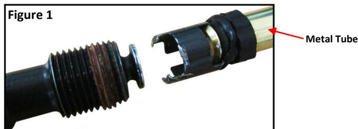
**Operation:** The friction nut has **left hand thread**. In that it makes light contact with the throttle sleeve, thrust washer.
